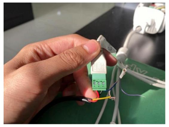
In this way we can power for mic by camera's reverse power supply, no need to power it alone.
